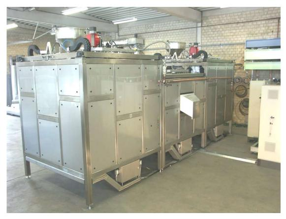
If the roasting time is longer than 6 minutes, two roasters could work at full capacity with a single cooler. This leads to a further reduction of the space required.
