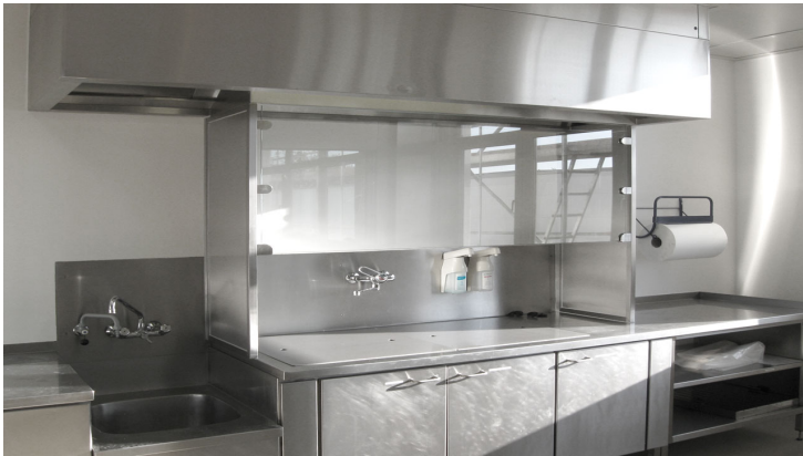
Laboratory workplace with suction, completely made from stainless steel.
