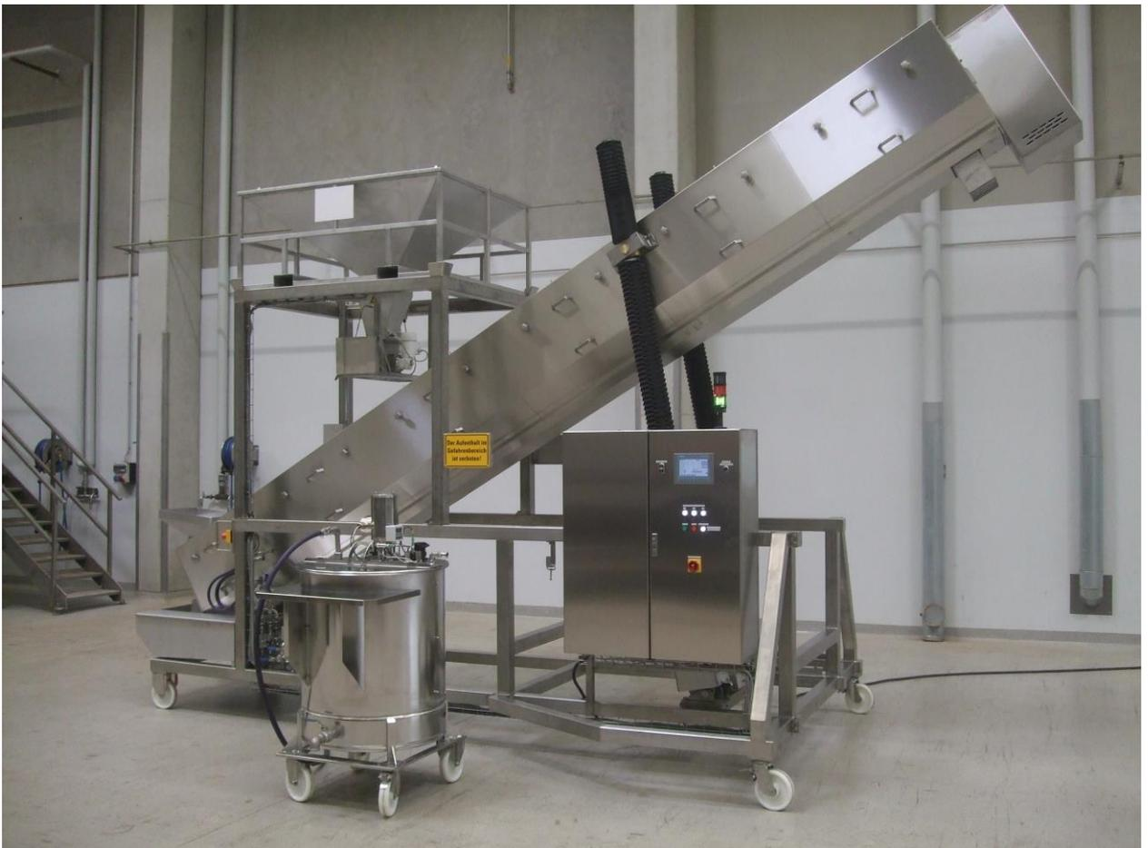
The mobile salting machine MSE-480 is a system for continuous salting with brine and for dry salting or coating of nuts and seeds before and after roasting with simultaneous vertical product transport.
